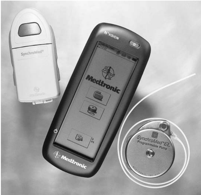
Fig. 8.6 Totally implantable intrathecal drug delivery system. Left to right: Personal programmer, a hand-held device that allows the patient to give a bolus intrathecally from the pump within preset parameters of dose and lockout time. Pump programmer that allows the therapist to set the intrathecal infusion parameters and check the volumes remaining in the pump at refill. Intrathecal pump with central filling port that takes a 22 G needle and meshed side access port that takes a 25 G needle and one-piece catheter.
